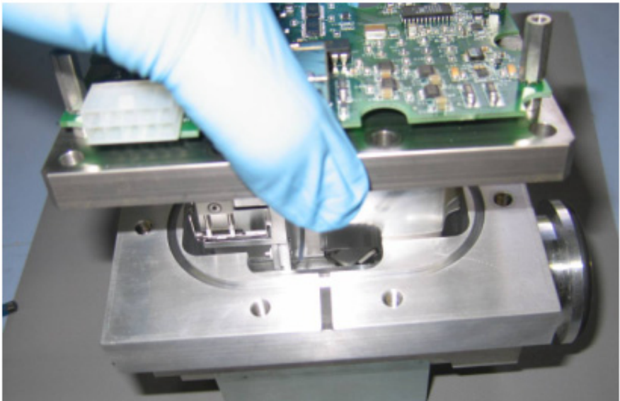
Figure 7: Spectrometer Assembly Removal
